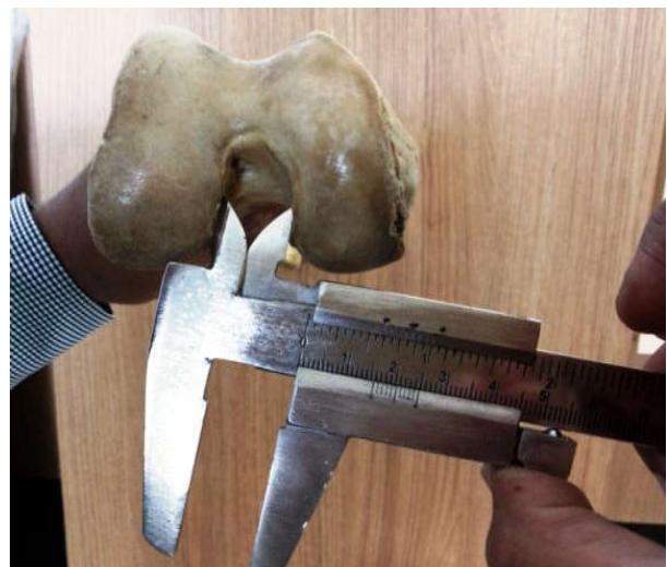
Fig. 3: Showing taking the transverse measurement of the intercondylar region of the femur using vernier caliper
